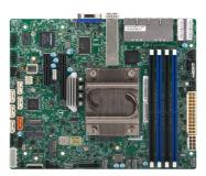
Embedded 8-Core Snow Ridge Intel OAT 8x 1GbE LAN 2x 25G SFP28,IPMI 2.0
