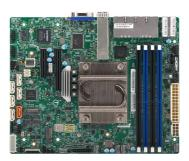
Embedded 24-Core Snow Ridge Intel QAT 8x 1GbE LAN 2x 25G SFP28,IPMI 2.0
