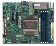
Embedded 16-Core Snow Ridge Intel QAT 8x 1GbE LAN 2x 25G SFP28,IPMI 2.0
