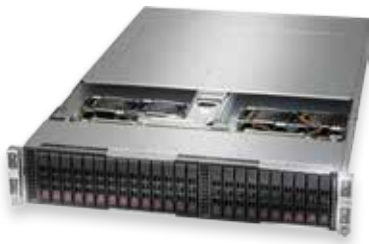
X11 BigTwin™ Quad DP Nodes, 24 SATA Drive Bays
