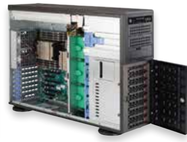
Mainstream 4U Standalone/Rackmount, 16 DIMMs
