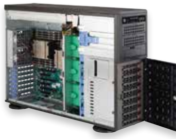
Mainstream 4U Standalone/Rackmount, 16 DIMMs
