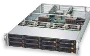
2U Ultra 3.5" Drives, NVMe, Titanium Level Power
