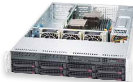
2U WIO 16 DIMMs, 6 PCI-E 3.0 x8 Dual 10G LAN
