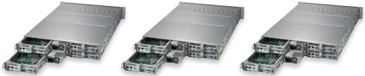
X11 TwinPro 2™ Quad DP Nodes, 24x 2.5" Drive Bays
