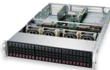
2U Ultra 24x 2.5" Drives, Titanium Level Power
