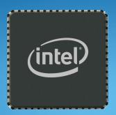
Low-power, small-footprint, single-port gigabit network controller with support for IEEE\* 802.1Qav Audio-Video Bridging for Desktop, Server, and Embedded applications.
