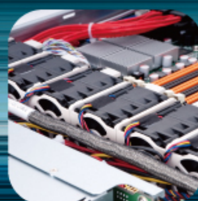
Up to 6 x middle 40 mm fans with anti-vibration design
