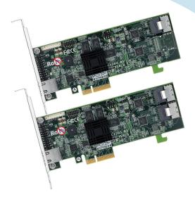
Stripe Size Migration, Global Online Spare, Automatic Drive Failure Detection, Automatic Failed Drive Rebuilding, Disk Hot-Swap, Online Background Rebuilding, Instant Availability/Background Initialization, Auto Reassign Sector, Redundant Flash Image and Battery Backup Module. The optional battery backup module provides power to the cache if it contains data not yet written to the drives when power is lost.
